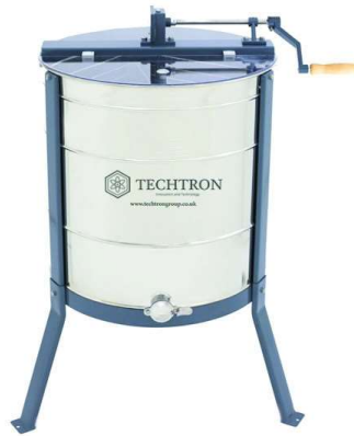
6/3 Frame Electric Tangential Extractor Ø 500 mm
