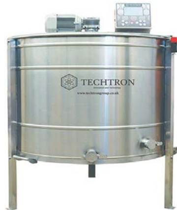
20/10 Frame Electric Cassette (5x2) Extractor Ø 950 mm
