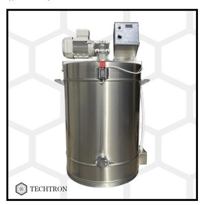
It is a model with a heater. In this model, the honey is heated by water flowing between the double walls of the container. The water is heated by electric heating.
