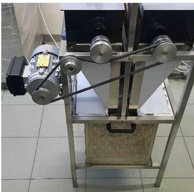
By releasing the screws that connect the motor with the construction, which is used as a belt crimper, you can unscrew the bolts of the bearing of the axels, and set the gap between the axel blades, for thicker or thinner honeycombs.
