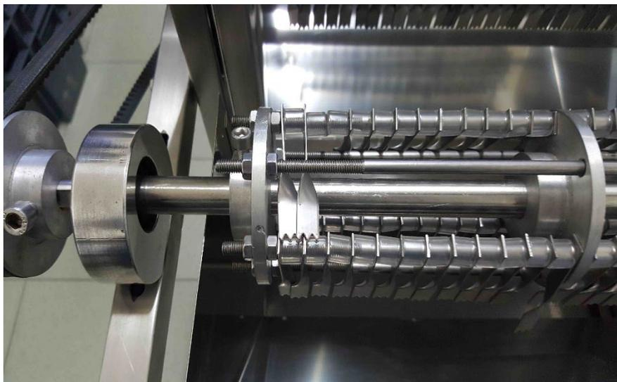
Once you do this, put the axel back and screw the bolts. Now the blade won't open when the equipment is in operation, and won't hit the frame.
